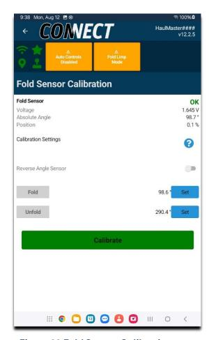
Figure 62 Fold Sensor Calibration
