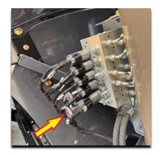
Figure 18 Auger Fold/Unfold Manual Valve
