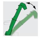
Using the pivot up joystick button ensure the auger moves in the pivot up direction as depicted. Using pivot down button ensure the auger moves in the pivot down direction as depicted. If controls are not behaving as intended please contact your local dealer.
