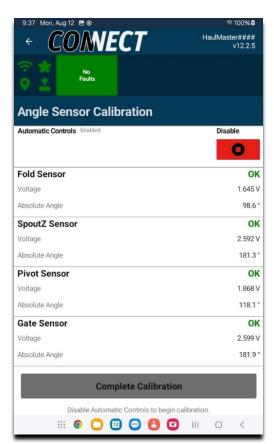
Figure 52 Angle Sensor Calibration
