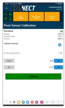
Figure 71 Pivot Sensor Calibration
