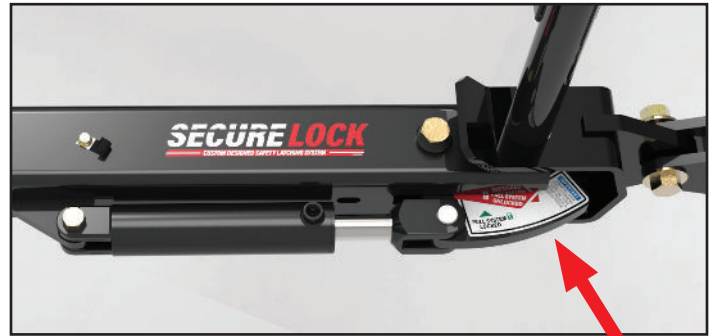
Figure F - Secure Lock not completely latched.
