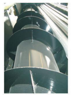
The tough 26" floating auger and 5" flighting delivers smoother higher volume feeding for today's large capacity combines.
