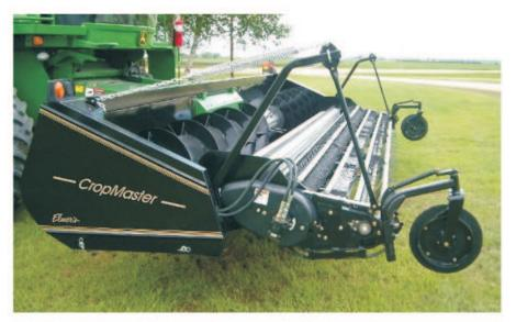
The 9 bar Pick-Up gently lifts and conveys your swath to minimize shatter in crops such as canola and edible beans. In uneven terrain, the torsion flex system follows the ground to pick up all the crop. The CropMaster Head and Elmer's Pick-Up, designed to harvest when you are ready.
