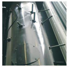
Fall-out protection steel, or alternate composite fingers prevent combine rotor damage.
