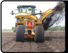
The Narrow Stance Kit has the wheels set directly behind the Wolverine ditcher, allowing for steeper angled ditches and allowing the ditcher to stay within the parameters of the waterways.
